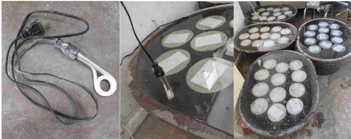
Hot wet environment (Relative humidity 100% and Temperature 29 \pm 1 °C)
