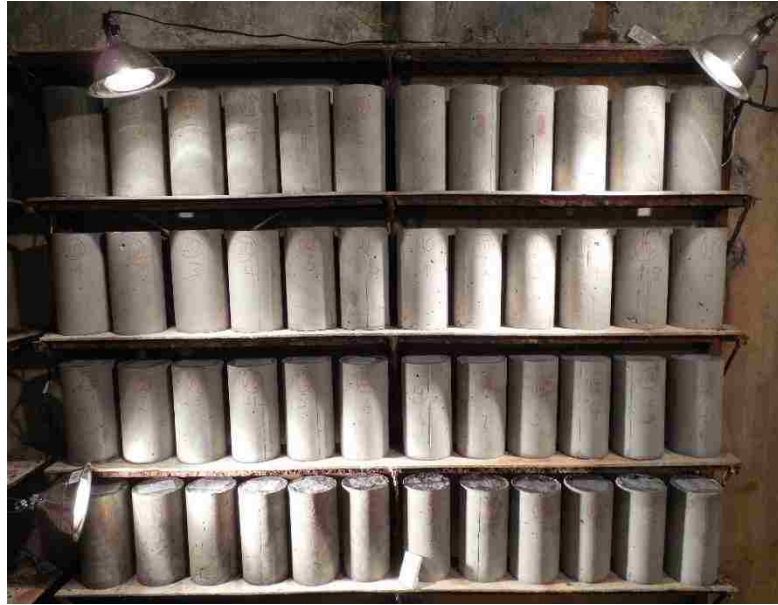
Hot dry environment (Relative humidity 20% and Temperature 29 \pm 1 °C)
