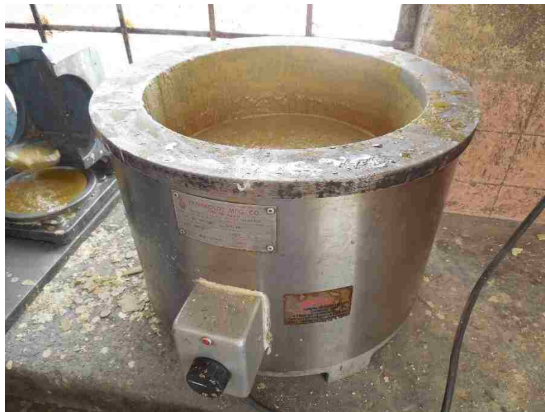
Sulfur mortar for capping concrete samples
